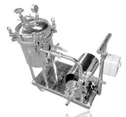
In this type of filter product to be filtered is fed in the shell with the help of suitable pump, where in it flows into the filter plates placed inside. The product enters plates from peripheral holes, while the impurities are retained on filter media & clear filtrate comes out from bottom outlet.
